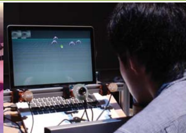
Eye tracking software and hardware that replaces the functions of the mouse with the movements of your eyeball.
